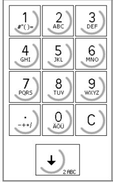
The alphanumeric keys have got more than one assignment. After pressing a key for the first time, the relevant first character, e.g. 'A' is displayed in the cursor position. After pressing for the second time, e.g. 'B' instead of 'A' is displayed; 'C' is displayed after pressing for the third time, etc. After the last signification, the first one is displayed again.
